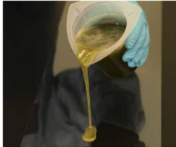
*After thoroughly mixing in the initiator, pour the resin onto the release film*
