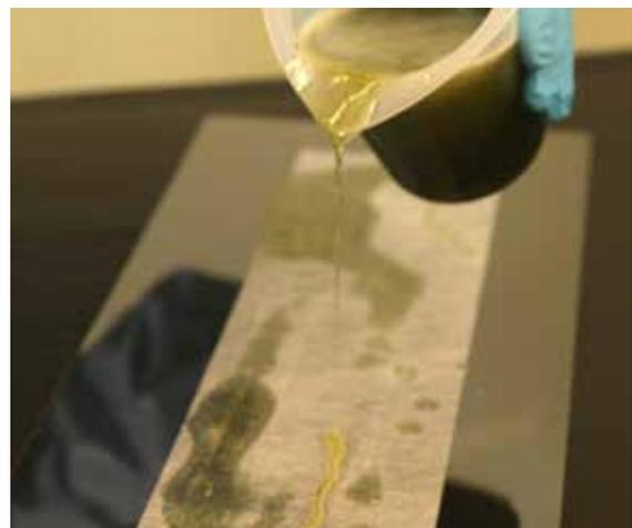
*Spread the resin over the entire fiberglass strip*
