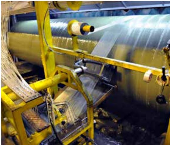
Filament winding process.
