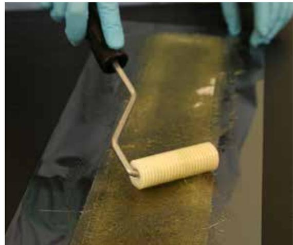
Work the resin into the second mat strip with a roller
