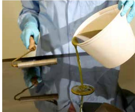
*Pour resin onto the release film*
