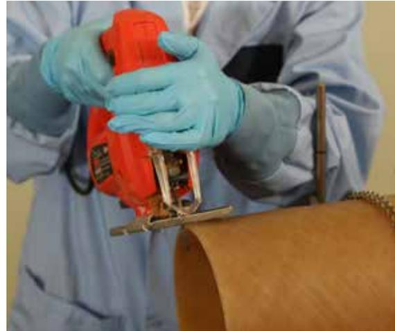
*Firmly support pipe sections; square the ends to be welded using a saber saw*
