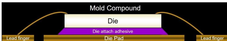
The semiconductor chip, also called a die (strange name, but as you will see, there are a lot of unique terms used in electronic packaging) is attached to the metal die pad with a filled-polymer adhesive called a die attach. The die pad and lead fingers are part of what is called a leadframe. The leadframe and die are encapsulated using a mold compound (black encapsulant in the image above). Mold compounds are highly filled epoxy resins.
