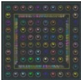
**Figure 7.** FOWLP test vehicle:  $4.1 \times 4.1 \text{mm}^2$ , with 72 balls on a  $0.4 \text{mm}$  pitch
