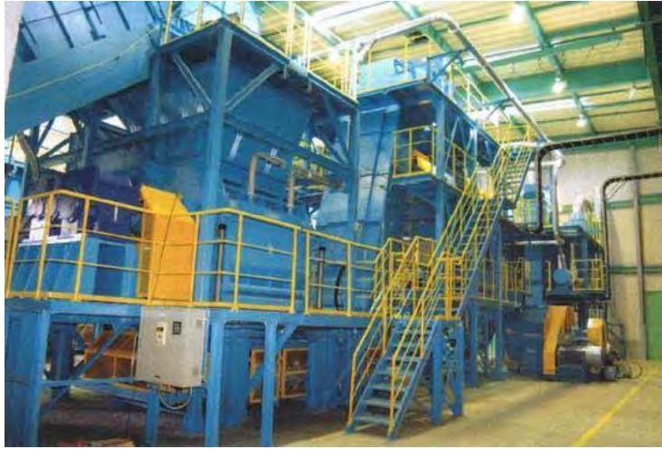
Figure 3.5: Typical pelletizing process facility (1 ton/h line)
