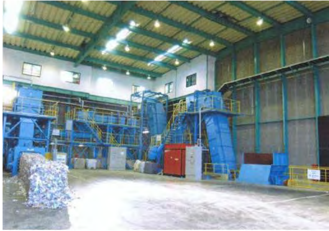
Figure 3.3: Example of pretreatment process (3 ton/h capacity)
