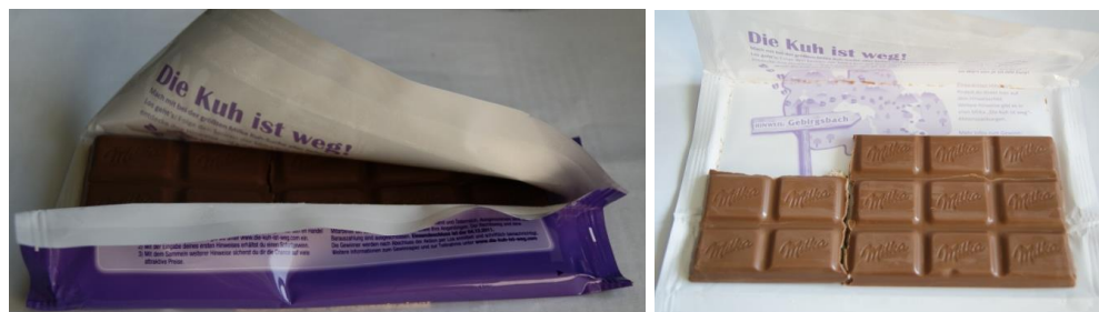
Figure 2 Chocolate packaging with printing on the food contact layer
