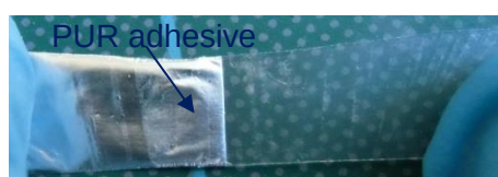
Figure 7 PUR adhesive sticks to the aluminium foil and partly also to the PA layer after separation
