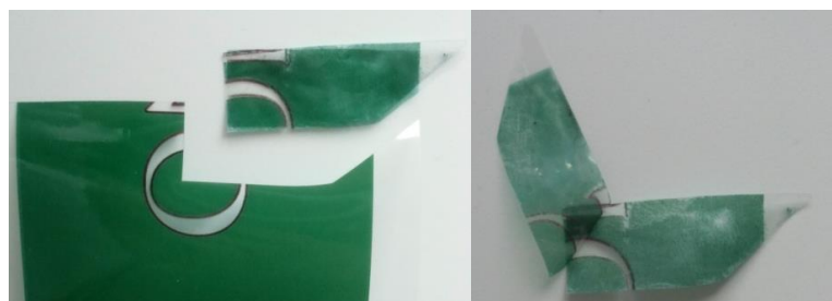
Figure 1 Laminate with reverse printing (PA/print/ PUR PE) after boiling in ethyl acetate for 2 min
