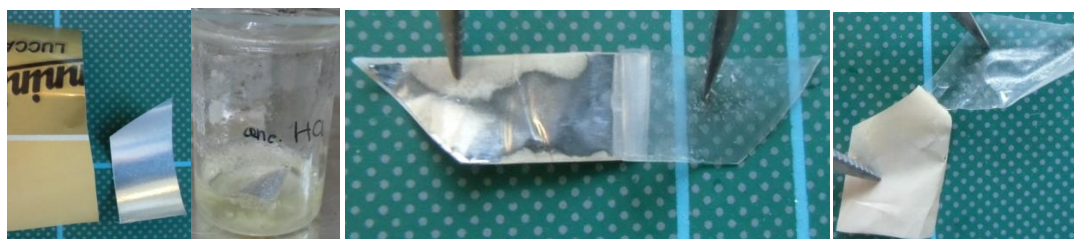
Figure 5 Sample with an inner aluminium foil before and after boiling in conc. HCl for 4 min (Al is partly dissolved) and 5 min (Al is completely dissolved)
