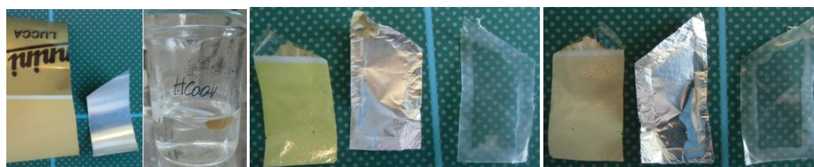
Figure 4 Sample (PET/print/ PUR Al foil/ PUR PE) before and after boiling in HCOOH for 5 min. Resulting 3 separated layers: PET/print, Al foil, PE (top and bottom view shown)
