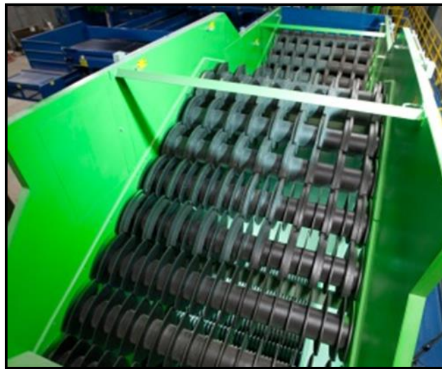
Figure 16 The Following is An Example of a Disc Screen
