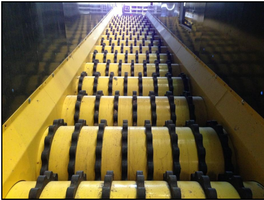
Figure 1 The Following is An Example of a Screen Designed for Anti-Wrapping
