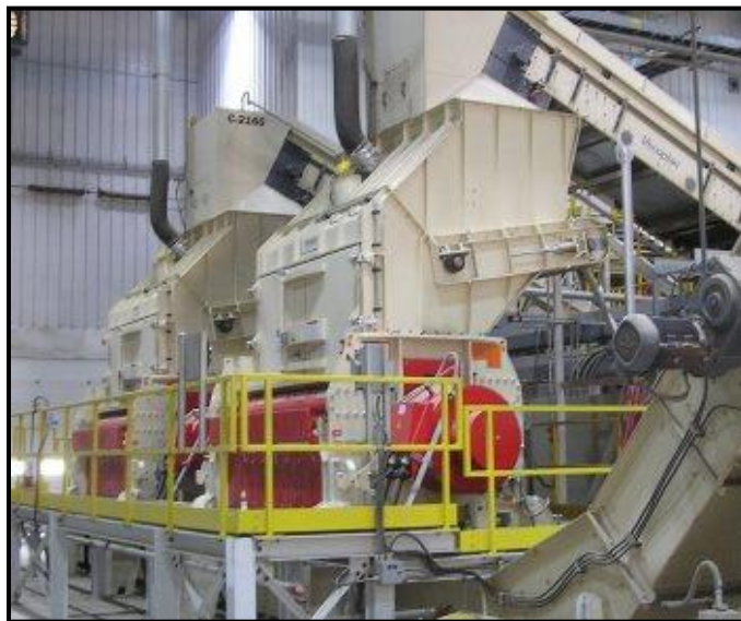
Figure 26 The Following are Examples of Secondary Shredders
